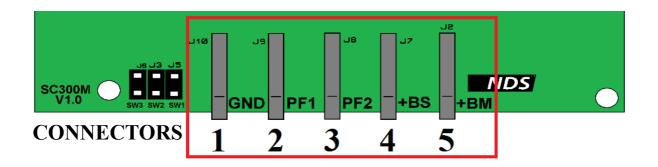
**PIN n°1:** Service Battery negative pole (GROUND) (and negative cable of the photovoltaic panels)
