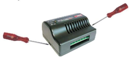
After removing the cover you have the full view of the PCB and the FASTON to connect the device to the solar panels and batteries; so you can also select the charging curve and replace the fuses (if necessary).
