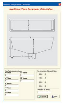
BEP's proprietary Window's based software application allows for TS1 senders to be programmed specific to tank shape, size and fluid type via a computer's USB port. Programming is a simple process and can be carried out by downloading free software from bepmarine.com and purchasing a programming kit TS1-PK.
