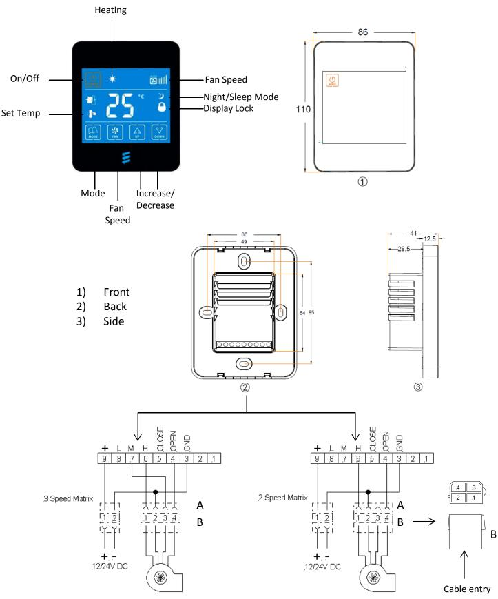
To wire a three speed matrix unit to plug B: Connect the high fan speed wire to pin 1 Connect the medium fan speed wire to pin 3 Connect the low fan speed wire to pin 4 Connect the matrix negative wire to pin 2 To wire a two speed matrix unit to plug B: Connect the high fan speed wire to pin 1 Pin 3 is not used Connect the low fan speed wire to pin 4 Connect the matrix negative wire to pin 3
