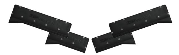
As a rule, the lift effect of a chine interceptor matches the lift of a straight interceptor one size larger mounted inboard of the chine, making them the go-to choice when selecting interceptors. Chine interceptors are particularly useful when transom space is limited abeam of outboards or sterndrives.
